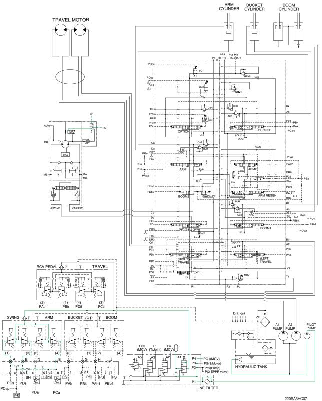
When the RCV lever (swing or arm in) is tilted, the pilot oil flows into SH port through shuttle valve. This pressure moves spool of the swing brake valve so, discharged oil from pilot valve flows to swing motor PG port. This pressure is applied to swing motor disc, thus the brake is released. When the RCV lever (swing or arm in) is set in the neutral position, oil in the swing motor disc cylinder is drained, thus the brake is applied.
