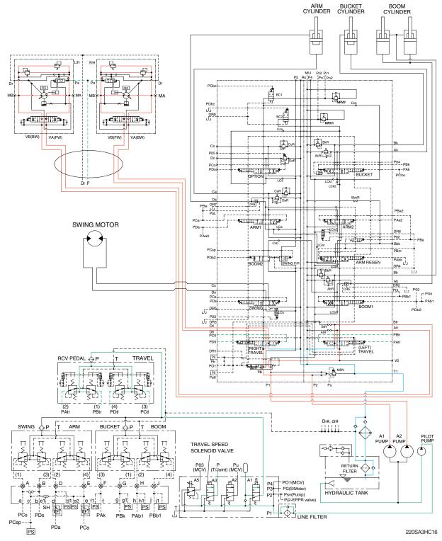
When the travel levers are pushed forward or reverse position, the travel spools in the main control valve are moved to the forward or reverse travel position by the pilot oil pressure (PAtr, PBtr, PCtl, PDtl) from the remote control valve.
